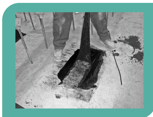
Figure 3 - Cohesive failure (pass)
